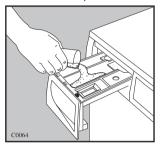
If required, pour fabric softener into the compartment marked \$\mathbb{8}\$ (the amount used must not exceed the "MAX" mark in the drawer). Close the drawer gently.
